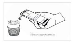
The NFC interface in the water meter is located above the display on the upper right side of the top of the housing.
