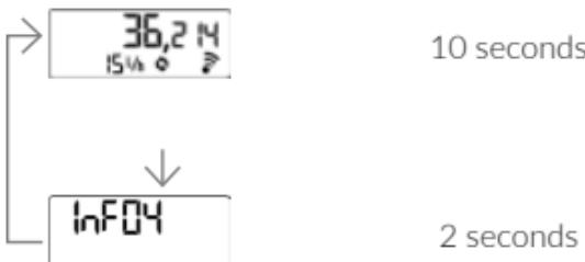
If the meter meets with an event or error, this is indicated by a message on the display. The event message display is integrated into the display loop for 2 second.
